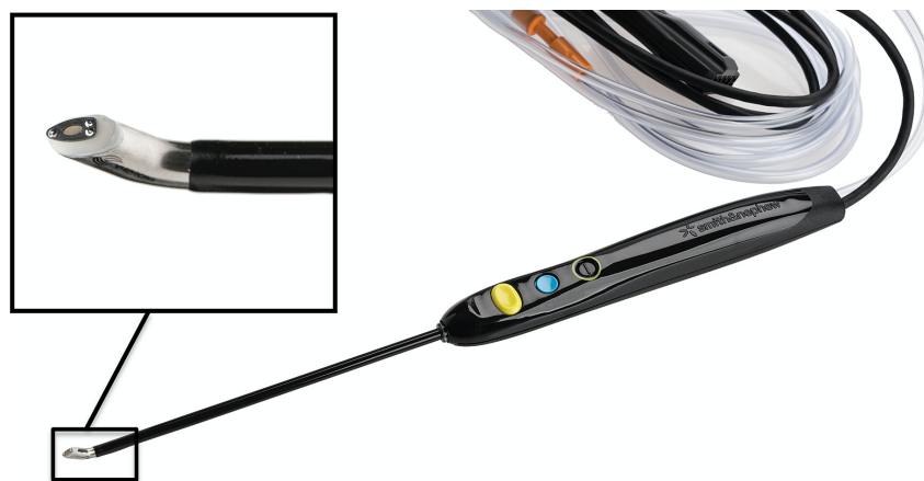
FIGURE 1: The Flow 50 RF ablation wand. The ceramic bevel at the tip of the wand allows the tip to rest on the joint surface without the electrode contacting the tissue. This design feature is aimed at improving the controlled introduction of target cartilage tissue into the stable plasma vapour layer adjacent to the bipolar electrode.
