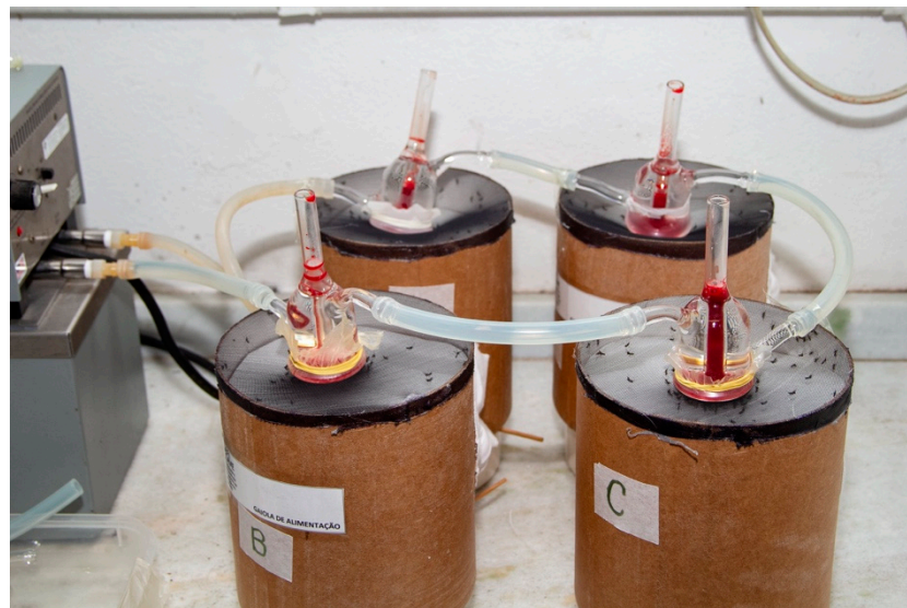
Figure 1. Artificial blood-feeding system for mosquitoes: four cages with retractable bottoms. Feeders filled with human blood are on top of the cages.
