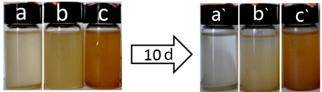
Figure 5. Digital photographs of the sedimentation of (a) raw mica, (b) mica ground at room temperature, and (c) mica ground at 200 °C.
