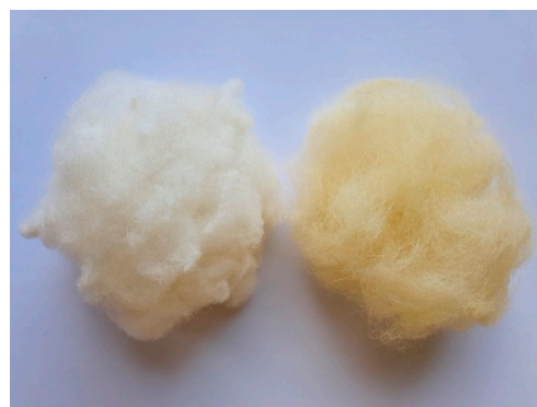
Figure 16. Photo of wool balls of the reference (left) and UV-aged (right) fibers.
