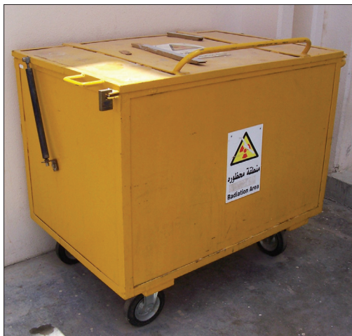
Figure 1: Temporary storage trolley in use for collection of solid wastes from I-131 wares in polythene bags. This trolley measuring 1.20 \times 0.85 \times 0.80\ \text{m} with castor wheels and locking facility, is anchored to the floor and is available at the waste collection yard, located behind the hospital premises
