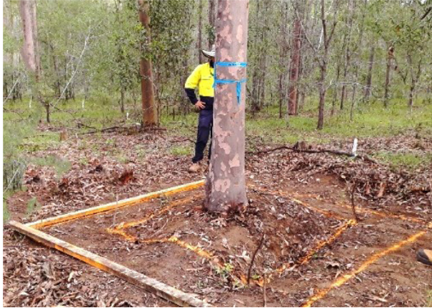
Fig. 5. Painted excavated area to define the limits of the excavation and the rootball monolith ( 1.5 \text{ m} \times 1.5 \text{ m} \times 1.0 \text{ m} deep; smaller square) containing the majority of the roots. Area around rootball monolith (larger square was 2.5 \text{ m} \times 2.5 \text{ m} ) was dug by an excavator to 1.0 \text{ m} depth. Any roots in this outer area were collected, before sampling the rootball monolith.
