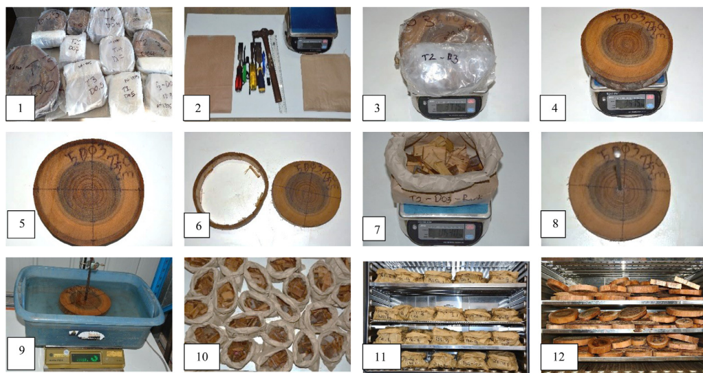
Fig. 7. Steps for measurement of stem discs in the laboratory: (1) defrosting discs, (2) tools to sample disc, (3) weighing disc inside the plastic bag, (4) re-weighing disc without plastic bag, (5) measuring bark thickness, sapwood and heartwood, (6) bark removed from the disc, (7) weighing fresh bark, (8 and 9) immersing disc for measurement wood density, (10 and 11) bark samples split into small pieces before being placed in paper bags and drying in the oven, and (12) drying discs in the oven.
