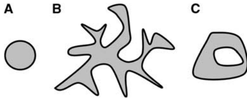
Figure 4 Three continuous objects: (A) simple disk, (B) a more complex tree-like structure, and (C) ring. Objects (A) and (B) are connected objects with one outside boundary and are therefore topologically identical. Object (C) contains a hole and is topologically different from the other two.
