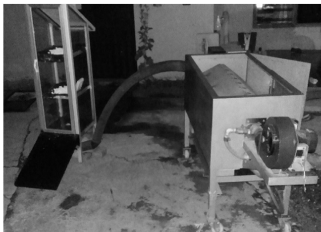
Figure 3. Hybrid solar-dryer system.
