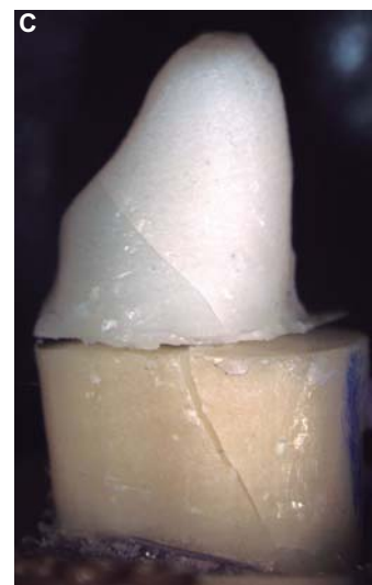
Figure 4- (A) Schematic diagram of the specimen positioned for the test, indicating the minimal thickness area (lingual portion) of the core where the fracture initiates. (B) Stereomicroscope representative image of specimen fractured in the mesiodistal direction (group C). (C) Root fracture associated with core fracture (group addition silicone) after the fracture resistance test
