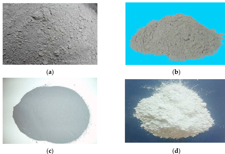
Figure 3. Raw materials: (a) fly Ash, (b) slag Powder, (c) silica Fume, and (d) stone Powder.
