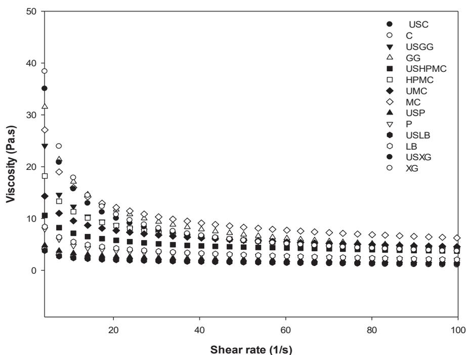
**Fig. 2.** Changes in apparent viscosity of batters formulated with different ultrasonic treated hydrocolloids. US – Ultrasonicated; C – Control; P – pectin; GG – guar gum; LB – Locust bean gum; MC – methylcellulose XG – xanthan gum; HPMC – hydroxypropyl methyl cellulose.
