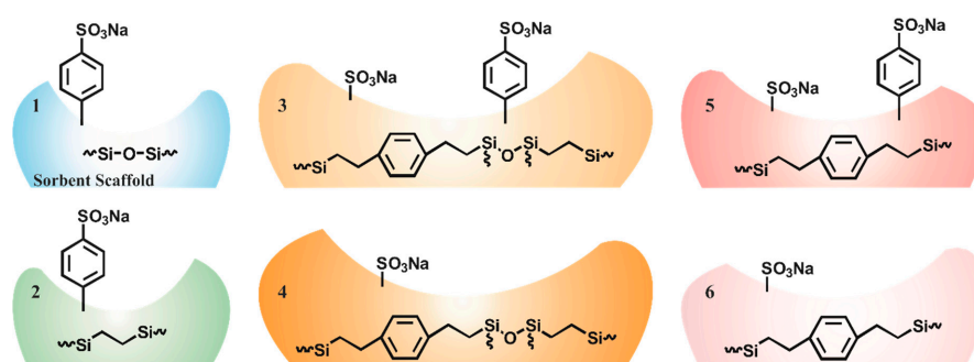
Figure 1. Glycerol sorbents. Schematics of the material variations are presented here showing both the groups within the sorbent scaffold (shaded area) and the groups added during post-synthesis processing. The numbers identify the type (1 through 6) and are used in the text to describe the sorbents as well as in the sorbent names. For example, S65-Ph(1) is a Type 1 sorbent while E50-Ph(2) is a Type 2 sorbent.
