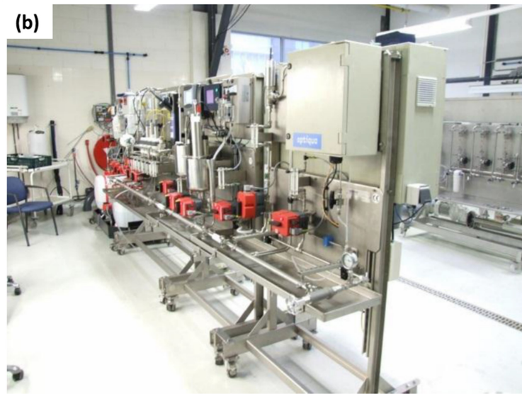
Figure 7. EventLab for online chemical event sensing. A new monitoring concept to continuously monitor the refractive index (RI) in real time is developed. RI is considered to be an indicator of the full spectrum of possible chemical contaminants and EventLab can be used as a highly sensitive (PPM level) generic optical sensor and an early-stage chemical contaminant warning system. (a) Schematic of the MZI chip used for measuring RI; (b) photograph of the optofluidic system installed in water plants for monitoring sodium chloride and so on [57].
