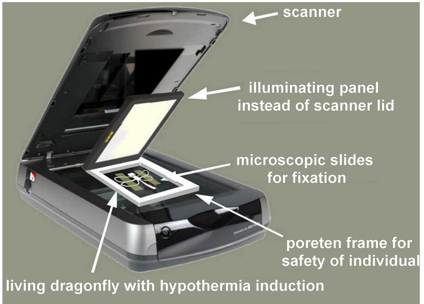
Fig 2. Method used to scan a living specimen with a desktop scanner.
