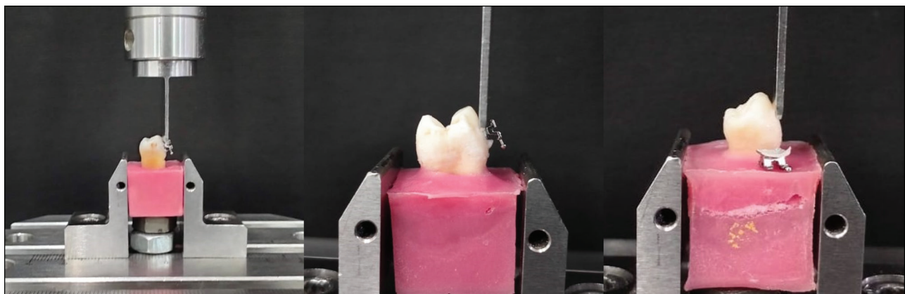
Figure 3: Shear bond strength evaluation using a universal testing machine
