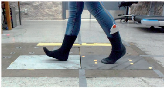
Figure 2. Participant walking over the force platforms while wearing the insoles in socks. Note that only one foot is placed on each platform, which allowed for a direct comparison between the insole on each foot (left and right) and the corresponding platform.
