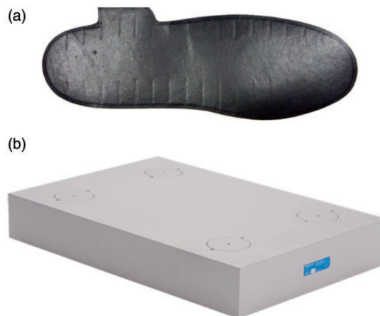
Figure 1. (a) The Medilogic pressure-measuring insole. (b) The Kistler 3 D force plate. 31
