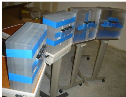
FIG. 3. Setup of EPD irradiation with backscatter from PMMA per ANSI/HPS N13.11-2009. The EPDs are located 120 cm away from the radioactive source and 108 cm above the floor.
