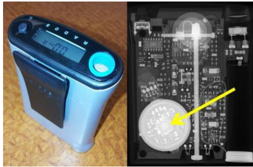
FIG. 1. RAD-60R (left) and radiograph (right). Arrow indicates the PIN Si-Diode.
