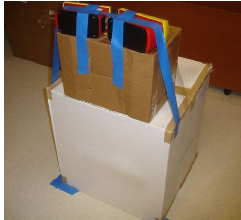
FIG. 4. Setup of ionization chambers for exposure-rate measurements concurrent with EPD irradiation. The ionization chambers are located 120 cm away from the radioactive source and 108 cm above the floor.
