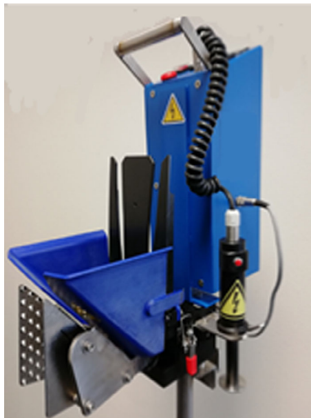
Figure 6: Head-to-body electrical killing device. Source: Top-equipment B.V.
