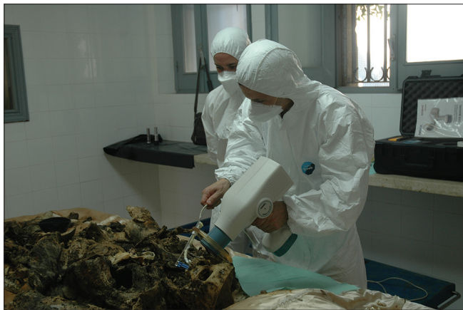
Figure 2: The portable radiographic unit (Nomad Examiner, Aribex Inc., USA) associated with a sensor for digital radiography
