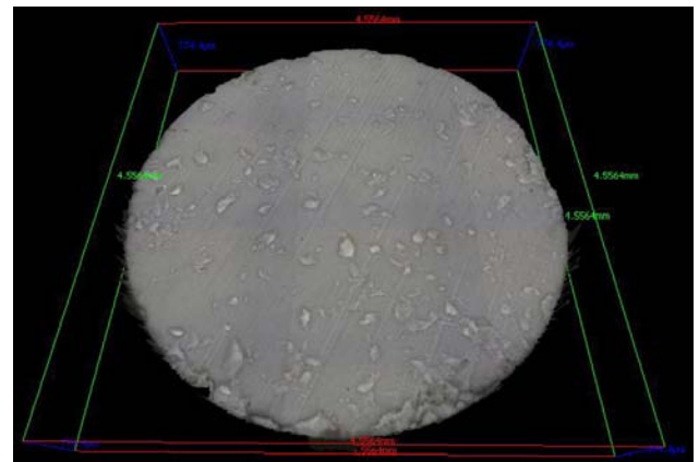
Fig. (1). Alicona image of a Sponceram HA carrier as used in this investigation. The defects are most probably due to cracking along some large agglomerates formed during calcinations of the porcine bone (each scale bar = 4,55 mm).
