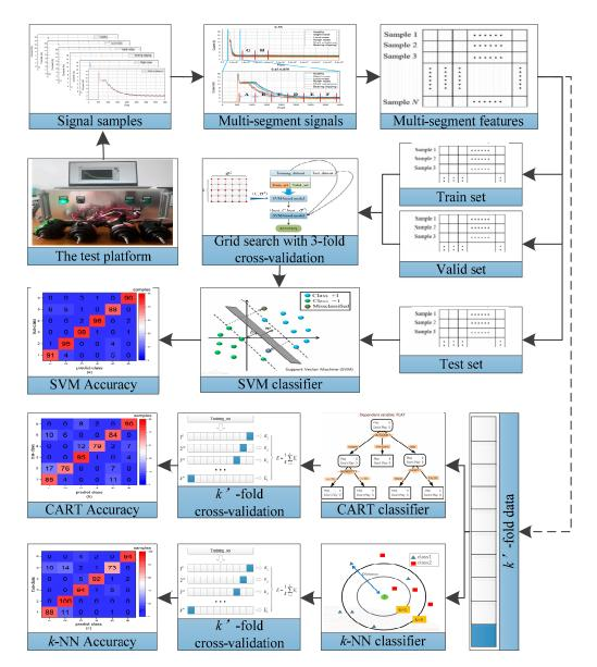
**Figure 3.** Fault diagnosis procedure of PMDCMs based on the SVM, CART, and *k*-NN by multi-segment features.
