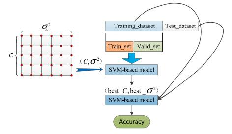
Figure 5. Parameter optimization of SVM for fault diagnosis of PMDCMs.
