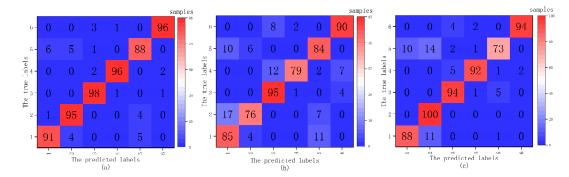
**Figure 7.** Confusion matrices of the three fault diagnosis models ((**a**) SVM-based model, (**b**) CART-based model, (**c**) *k*-NN-based model). The *x*-axis corresponds to the predicted labels, while the *y*-axis represents the true labels.
