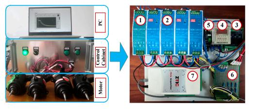
Figure 4. The fault diagnosis platform for PMDCMs.
