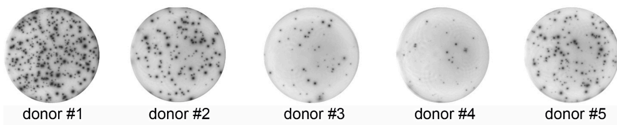
Figure 1. Exemplary images (collected using QuantiHub 4.1 ELISPOT reader) of IFN \gamma -formed spots by PBMCs isolated from five different donors. The same number of cells from different donors was plated per well and cells were stimulated with the same mitogens for the same period of time. Notice the significant donor-to-donor differences in the spot-forming activity of PBMCs.
