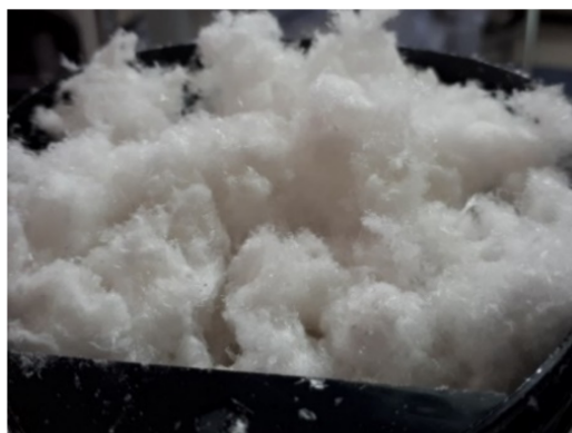
Figure 8. Hydrolyzed collagen obtained in the following conditions: type of enzyme: Papain; E/S: 1/20; time of hydrolysis: 0.5 h).
