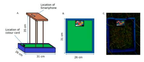
**Figure 2.** Schematic overview of the imaging rig. (**A**) Lateral view. (**B**) Top view. (**C**) Field image taken using the rig. The blue surround of the image facilitates removal in pre-processing, whilst the colour card provides an internal standard.
