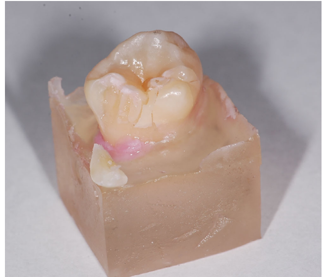
FIGURE 2 Fractured tooth with chipping of the enamel wall along the dentin core (1)
