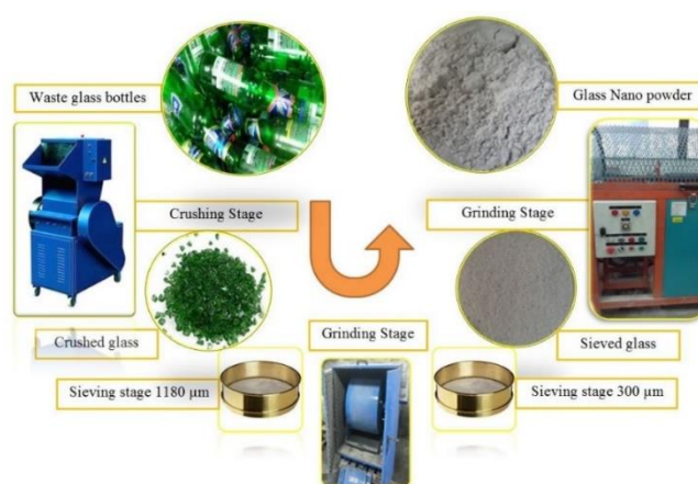
Figure 1. BGWNP preparation stages.
