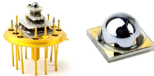
Figure 57. The photodetector assembled on the 3-stage Peltier thermoelectrical cooler and GaAs immersion microlens. The improvement in detectivity reached by hyperhemispherical microlens is proportional to n_r^2 , where n_r is the GaAs refractive index (after [180]).
