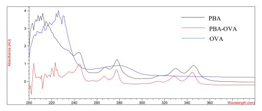
Figure 2. UV spectrum of OVA, PBA and PBA-OVA.
