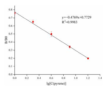
Figure 4. Standard curve for PYR in the ic-ELISA.
