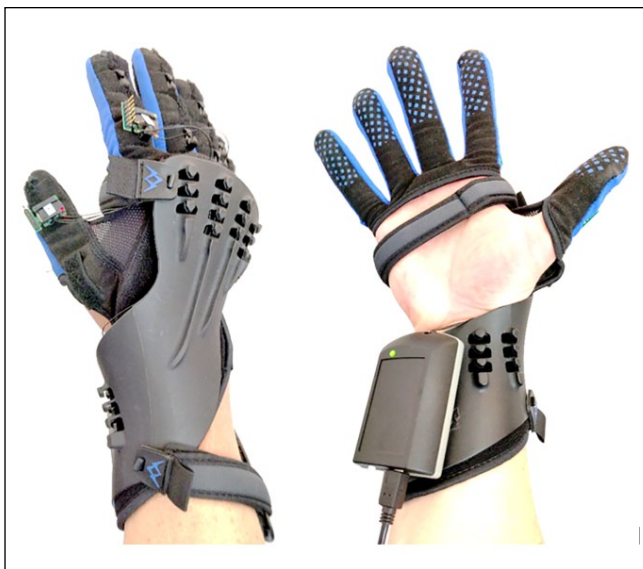
Figure 1. SaeboGlove orthosis with sensors to track grasp interactions.
