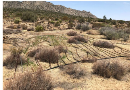
FIGURE 2 | (A) Field experimental layout of our research site (adapted from Krichels et al. 2023b). (B) Plastic roofing was used to exclude precipitation in Winter- and Summer- plots and (C) irrigation lines to add precipitation to Winter+ and Summer+ plots.
