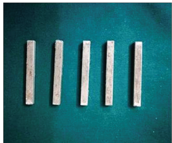
Figure 1: Metal bars of dimension 50mm × 6mm × 4mm used for mould space preparation according to specifications provided by American Dental Association (ADA)
