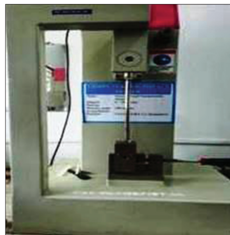
Figure 7: Izod/Charpy Impact Tester used for evaluation of impact strength of prepared acrylic samples
