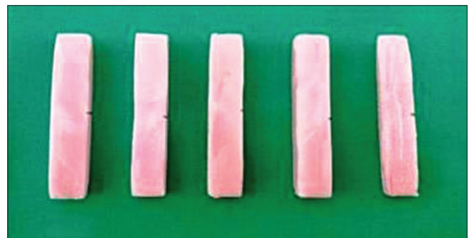
Figure 3: Prepared acrylic samples for evaluation of impact strength in impact testing machine
