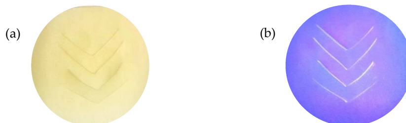
Figure 3. Photograph of LC films for solid sample fluorescence analysis (a) film under visible light, (b) film under UV light.
