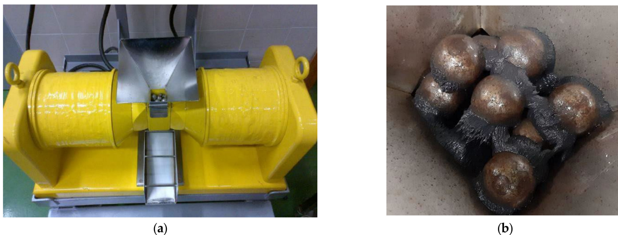
Figure 1. Magnetic separation tests at WHIMS: (a) separating equipment, (b) magnetic product retained in the matrix.
