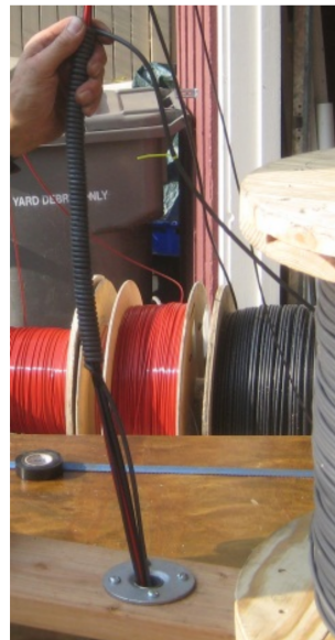
Figure 3. A wrapped section, or heating “dot,” on the cable assembly. In the background the two spools of red fiber optic cable are seen, and to the right, the heavy power feed cable, and to the far right the vertical spool of wrapping cable which was on a rotating holder that allowed wrapping around the other four cables (the linear heating cable spool is not visible).
