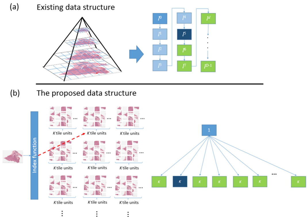
Figure 6. The difference between the existing pyramid data structure and the proposed tile units structure. The size of a set in the existing data structure requires l^d , where d is the depth of the tier. Compared with existing pyramid data structure, the size of a set is limited at most K tiles (i.e. 2^8 ).
