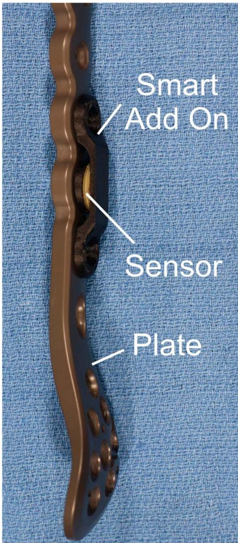
**Figure 2.** “Smart” plate with sensor and add-on plate attachment.
