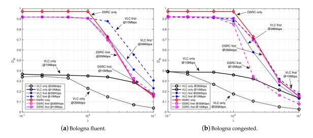
**Figure 6.** Delivery rate vs. packet generation rate with 1-DSRC and 1-VLC varying the data rate of VLC in fluent (**a**) and congested (**b**) traffic conditions.
