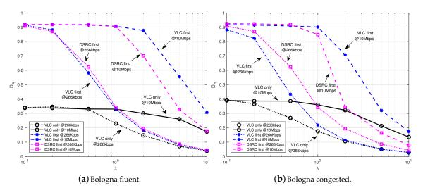
**Figure 5.** Delivery rate vs. packet generation rate with 1-VLC varying the data rate of VLC in fluent (a) and congested (b) traffic conditions.
