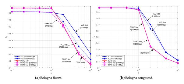
**Figure 4.** Delivery rate vs. packet generation rate with 1-DSRC varying the data rate of VLC in fluent (a) and congested (b) traffic conditions.
