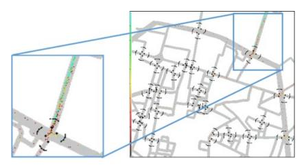
**Figure 8.** Congested traffic scenario with 23 VLC RSUs at 10 Mb/s. Colors of vehicles indicate the number of packets in the on board queue (light blue = no packets in the queue, black = full queue).
