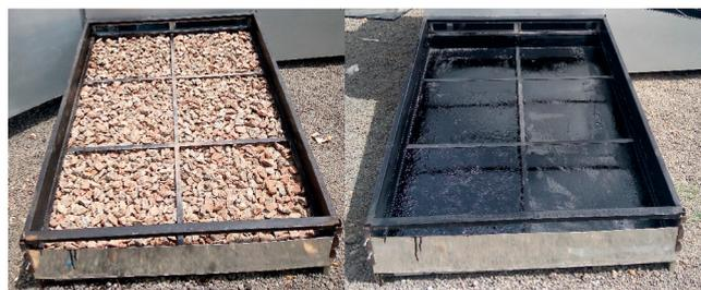
Figure 3. Photograph of a solar dryer collector with and without TES.
