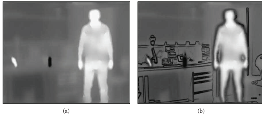
FIGURE 13: Visually enhanced IR segmentation. The base IR image (Figure 5(a)) above is smoothed with the anisotropic method (a) and then cartoonised via edge overlay from the visual scene (b).
