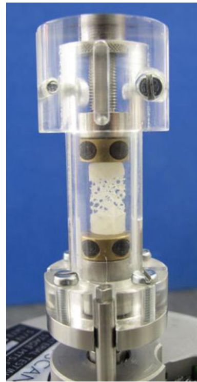
FIGURE 1. A cement–augmented specimen inside the compression stage used during \mu CT imaging.
