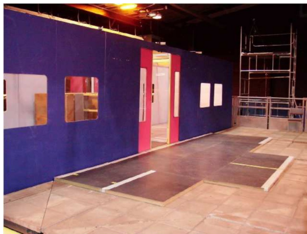
Figure 1. Pedestrian Accessibility Movement Environment Laboratory (PAMELA) configured as a London Underground carriage to study effect of door width and vertical gap [12].
