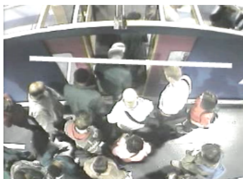
Figure 9. Counting setup: an imaginary line on the image is considered and the tracking results are used to count people crossing the line up (boarding) or down (alighting).
