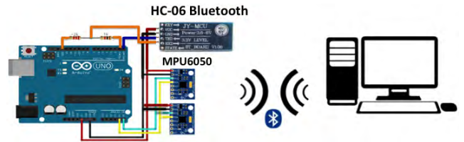
FIGURE 1. Experimental Instrumentation, the kinematic signals obtained by two MPU6050 inertial sensors were acquired with an Arduino UNO platform and transmitted via Bluetooth (HC-06) to a personal computer.
