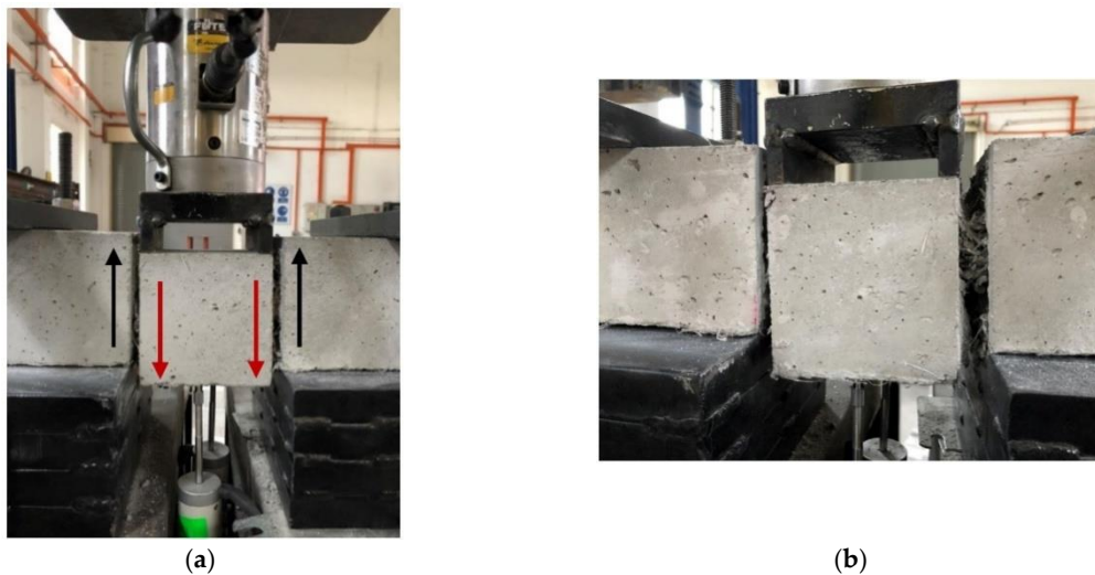
Figure 8. Experimental photos showing the (a) in-plane shear (mode II fracture) failure and (b) specimen instability due to higher fiber count on the right-hand side of the prism.
