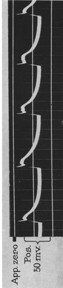
FIG. 1. Successive similar action curves. The spot recorded was in contact with 0.009 M NaCl + 0.001 M KCl and was connected to a spot in contact with 0.01 M KCl which kept the P.D. constant approximately at zero. Since the location of the zero is not exact the figure is marked "App. zero."
