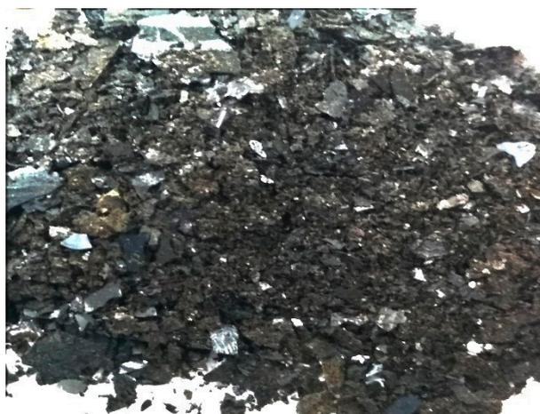
**Figure 1.** Black and shiny appearance of the asphaltene extracted from thermally treated COTBS.
