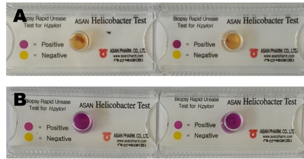
Figure 1. Gross findings of rapid urease test with CLO test kit. (A) Negative reaction (yellow color change) with control mice. (B) Positive reaction (red color change) with H. pylori infected mice.
