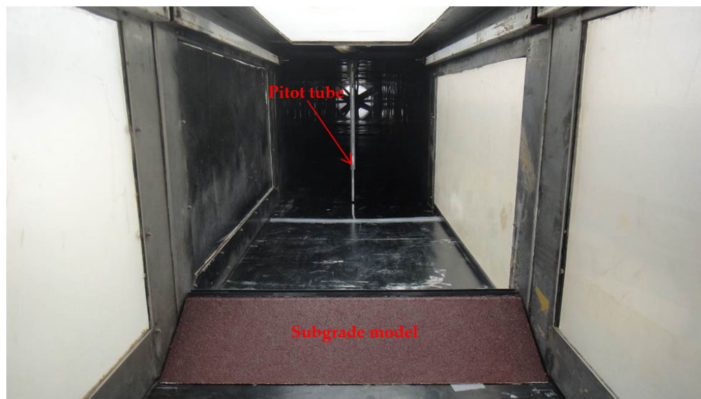
Figure 3. Subgrade model for the wind tunnel experiment.
