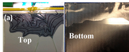
(a) Top and bottom surface showing large dry spots on the laminate infused with no flow mesh
