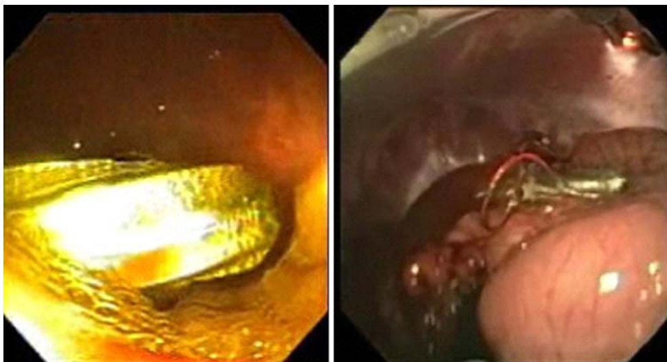
Fig. 5 The 12 mm mobile robot successfully traverses within the gastric ( left ) and peritoneal ( right ) cavities
