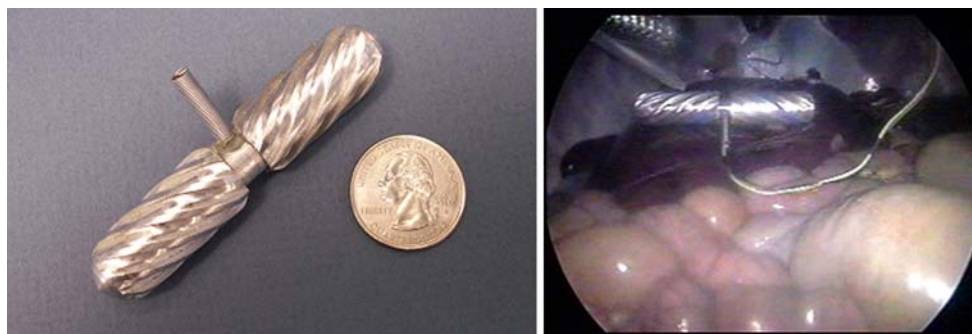
Fig. 2 The 15 mm mobile robot ( left ) successfully navigates within the peritoneal cavity ( right )
