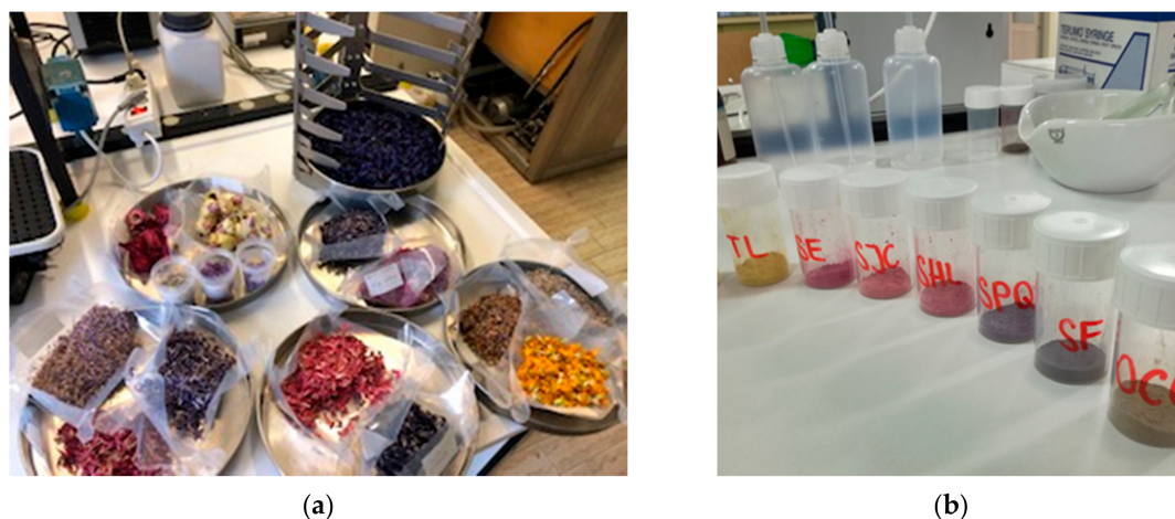
Figure 2. Two of the steps of sample preparation. (a) Samples after freeze-drying; (b) Samples after homogenization performed in 25 mL Teflon grinding jars with zirconium oxide grinding balls (MM2 Mixer Mill, Retsch, Germany).
